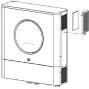
Step 3: Clean air filter foam and dustproof case. After clearance, re-assemble the dust-kit back to the inverter.
